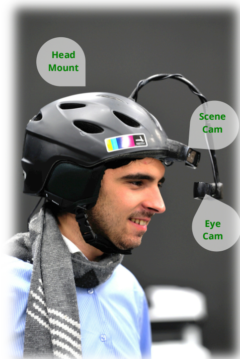
FIG I: Eye Tracker set-up
